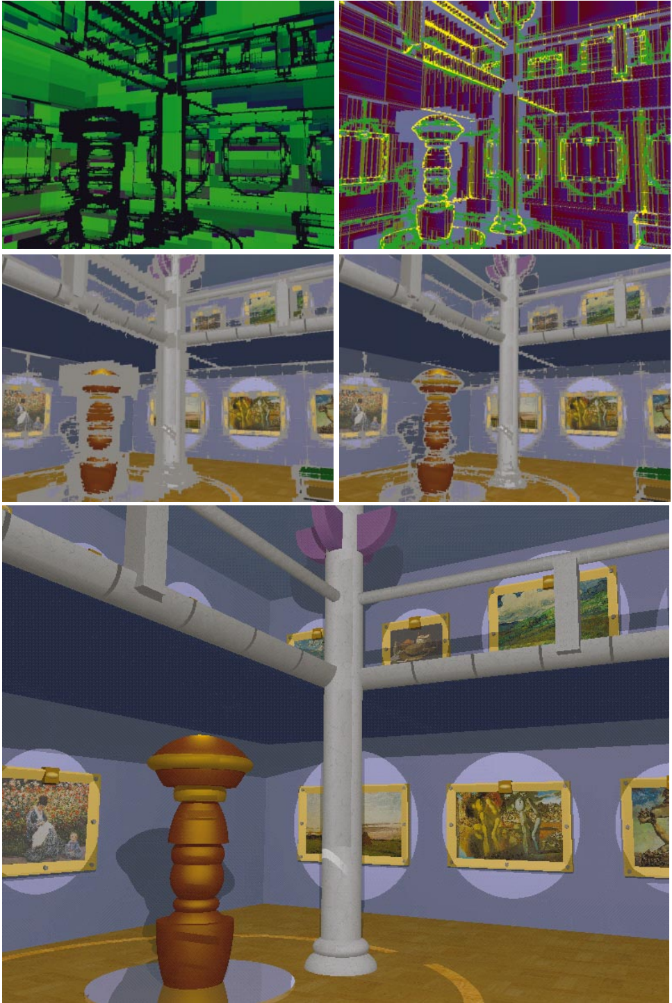
Fig. 21. Museum scene. Top row (left to right): reprojection buffer, color-coded image. Middle row: span-filled pixels, and span-filled and interpolated pixels; bottom: final image.
