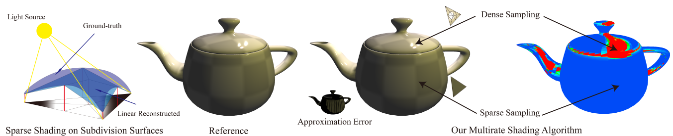
Figure 1: Ground-truth shading signals can be linearly reconstructed by shading values on the vertices of subdivision surfaces (left). The piecewise interpolation errors are analytically estimated to decide the optimal subdivision given an error threshold. We propose a multirate shading algorithm leveraging sparse piecewise reconstruction (right). High-frequency shading signals require dense sampling while low-frequency signals can be efficiently approximated by sparse sample points. Different shading rates (i.e., granularities of subdivision) are computed at runtime using our derived estimator.
