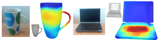
Figure 11: For real objects: we took a real mug and laptop, created 3D models of them, and computed the grasp saliency map for the mug and the press saliency map for the laptop.
