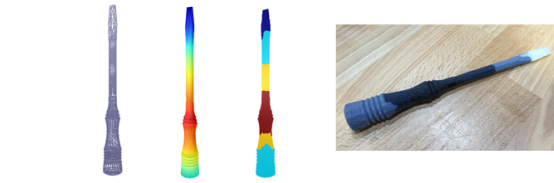
Figure 13: Fabrication Material Suggestion: 3D Printing. The more likely it is to grasp, the more soft the material to make it more comfortable to grasp. Input screwdriver mesh, grasp saliency map, saliencies discretized and blended into 4 clusters of volumetric parts, and screwdriver with 6 discrete parts and 4 suggested materials fabricated with an Objet Connex multi-material 3D printer.
