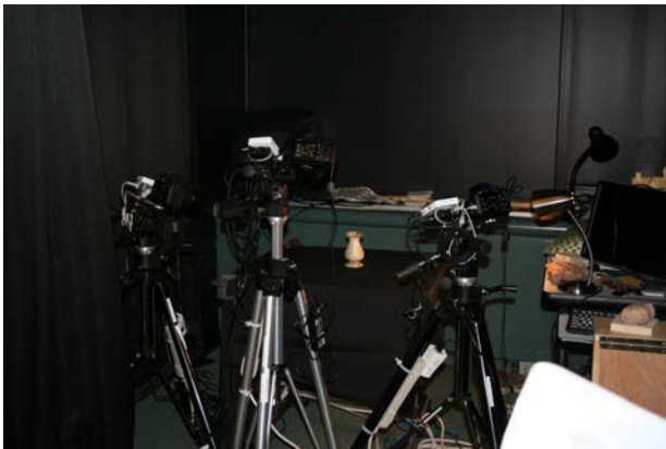
Figure 2. Our hardware capture setup consists of three projector/camera pairs.
