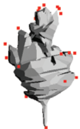
6 A sample output of the automatic selection algorithm. Voronoi nodes near the red points in the figure will be marked for the medial axis approximation algorithm.
