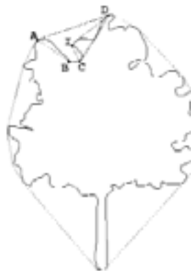
5 Determining interesting 2D vertices. ABCD is a first-order convex hull and CID is a second-order convex hull. I is an interesting vertex on an even-order convex hull and corresponds to a visible branch tip.
