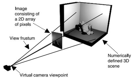
Figure 1—A 2-D image is defined by specifying a virtual camera and the lighting, shape, and materials in a 3-D scene.
