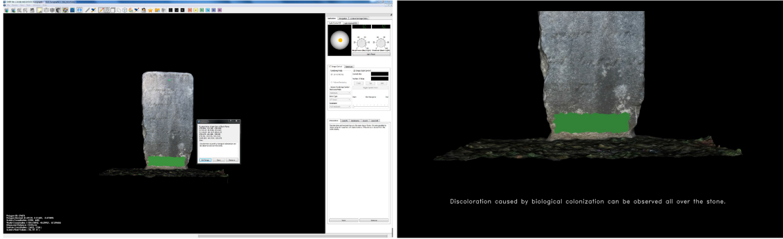
Fig. 12. 3D animation scheme for frustum notes (left: CHER-Ob interface, right: video frame). The camera looks toward the note's center from a distance and rotates around the object with subtitles at the bottom.
