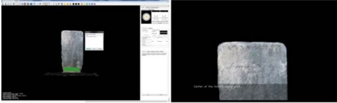
Fig. 10. 3D animation scheme for point notes (left: CHER-Ob interface, right: video frame). The camera looks toward the note's center from a distance along the triangle normal with subtitles at the bottom.
