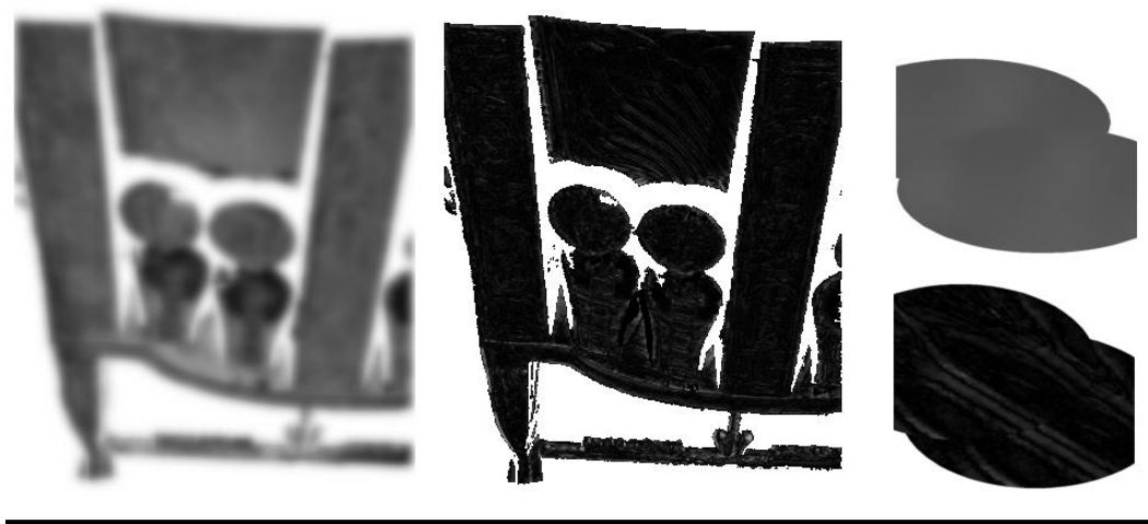
Figure 8. Left: Low frequency component of “unlit” image, Middle: High frequency component of “unlit” image, Right: All low frequency images blended smoothly in final image (top, high frequency component from only one input image in the final image(bottom)).
