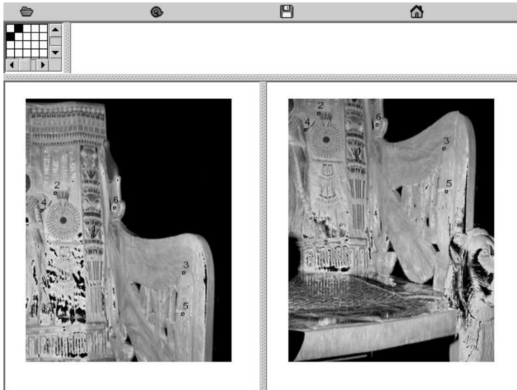
Figure 5. Range scans represented as images for picking corresponding points, shown with corresponding numbers here. In the upper left hand corner is a matrix visualization of scans that have been matched .
