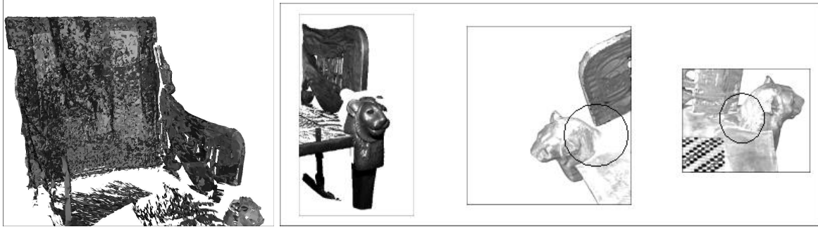
Figure 6. Left: A set of aligned meshes shown to inspect quality of initial tree of related meshes. When viewed in full color meshes which do not interleave well with surrounding meshes stand out. Right: It was impossible to obtain shape scans at the back of the lion's head. These sections had to be rebuilt by hand due to the failure of standard hole filling algorithms.
