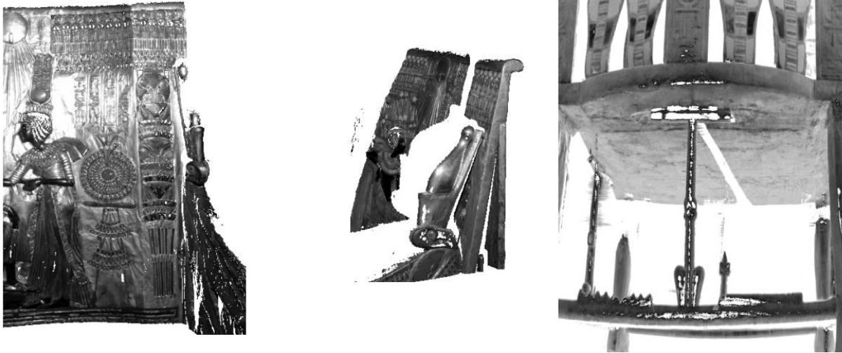
Figure 3. Two scans (left and center) on either side of a thin arm. These scans are shown in the form of projecting the scanned points into one of the color images obtained from the same view. These images were also used for scan cleaning. On the right, a scan of the bottom of the throne is shown, in the form used in Fig. 5 for registration. The curving of the lower run of the chair is an artifact of displaying the cylindrical scan as a rectangular image.
