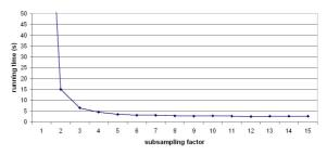
Figure 13: Speed-up due to downsampling for 17 segments and a 576x768 image. The value for the full-scale filtering is 173 sec.
